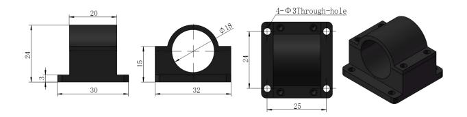
This simple mount acts as combined heat sink mount for 18mm diameter diode modules. Loosen the four small set screws and remove the top half of the module mount to put the laser in. The laser is held firmly by tighten the screws. The module mount reserved 4 through-holes for user to fix the laser on a flat and thermally dissipating surface.
