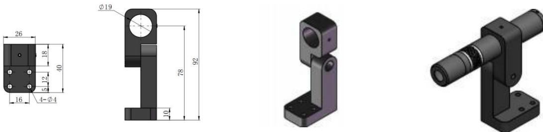
The module mount is used for 19mm diameter diode modules. Loosen the two small set screws on the top half of the module mount to put the laser in. The laser is held firmly by tighten the screws. The module mount base reserved the 4 holes for users to fix the laser on a flat and heat-dissipating surface. Moreover, the module mount can be tilted about 45°.
