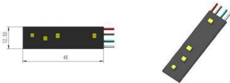
DIMENSIONS OF 5-12V PCB FOR MDL-SL SERIES LASER MODULE (mm):
