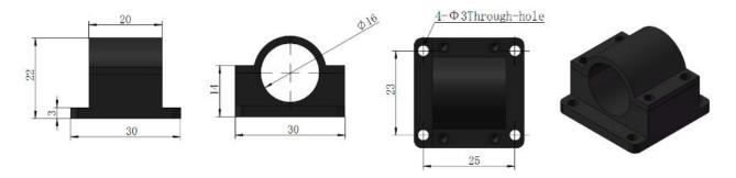
This simple mount acts as combined heat sink, electrical insulator mount for 16mm diameter diode modules. Loosen the four small set screws and remove the top half of the module mount to put the laser in. The laser is held firmly by tighten the screws. The module mount reserved 4 through-holes for user to fix the laser on a flat and thermally dissipating surface.
