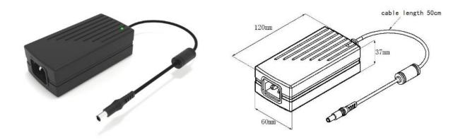
The Universal Diode Laser Module Power Supply with CE-marked provides a well-regulated 5 VDC. This auto ranging power module can be connected to any 85-264 VAC 47/63 Hz supply. There is an IEC 60320 input socket and a 0.5m output cable terminated with an easy connect/disconnect jack socket. The Headset connector which could also be found in accessories is compatible with the power supply jack.
