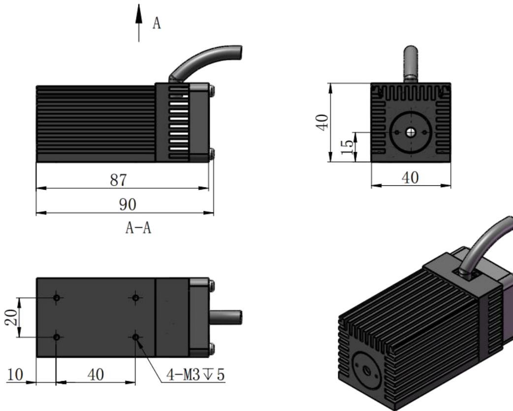
Dimensions of PSU-V-OEM power supply
