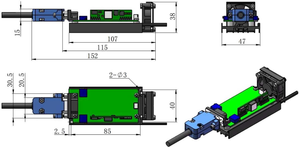
Dimensions of PSU-V-OEM and PSU-I-OEM power supply with dust cover(110×70×47mm<sup>3</sup>)
