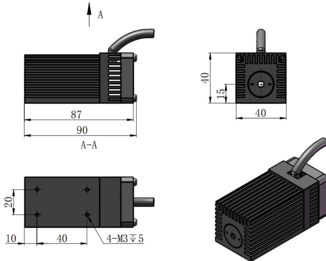
Dimensions of PSU-V-OEM power supply
