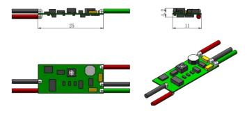
Dimensions of external PCB2(wide voltage input range, 20×30mm<sup>2</sup>, 5-12VDC, TTL and Analog)
